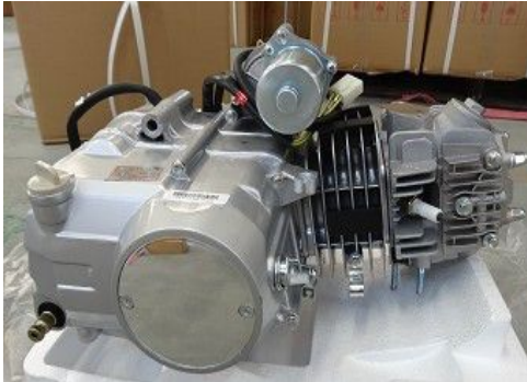
125cc engine (aluminium cylinder, kick & electric start, manual / automatic clutch)
